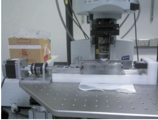
Fig. 6.4. Horizontal uniaxial mechanical testing device mounted on the stage of the multi-photon microscope
